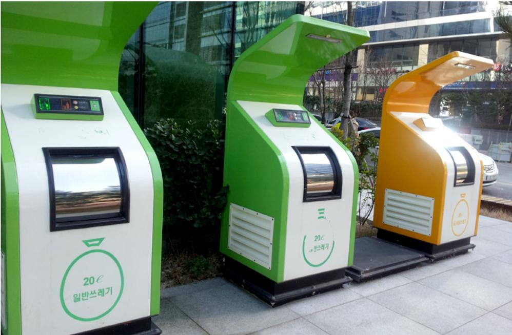
RFID-equipped waste disposal bins are used to automatically measure the weight of waste. Photo credit: Seoul Urban Solutions Agency.
