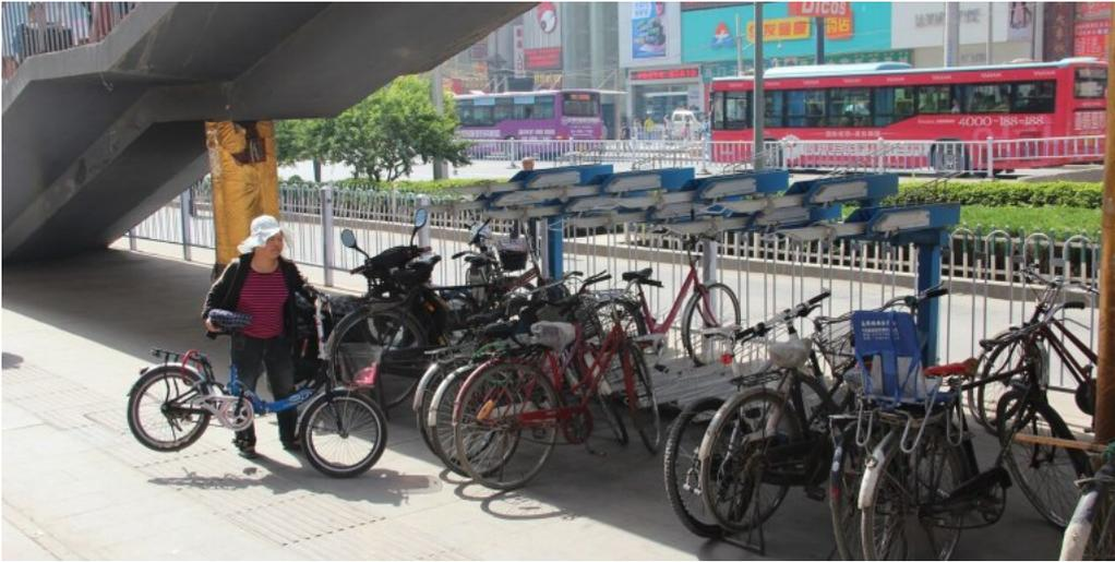
To promote the use of nonmotorized transport, the city provided dedicated 3.5- to 5-meter-wide bicycle access lanes between sidewalks and carriage lanes and bicycle parking facilities at the BRT stations. Photo credit: Lloyd Wright/ADB.
